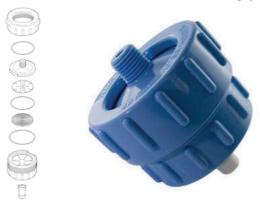
The GVS polypropylene 47 mm filter holder is designed especially for ultra cleaning and sterilizing liquids under positive pressure. In addition this holder can be used for aseptic sampling of liquids or gases at point-of-use or when samples must be collected and processed on-site.
