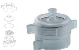
The GVS polypropylene 25 mm filter holders are very useful for ultra cleaning and sterilizing small volumes of liquids from a syringe. Due to the polypropylene construction, they can be used over a wide temperature range with excellent chemical compatibility. In the case of the syringe, the inlet cap locks into the base to prevent twisting damage to the membrane as the cap is tightened. Projection lugs on the base and the cap allow these units to be assembled and sealed quickly and efficiently.
